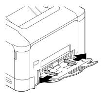
3 Push up the center of the flip-top plate until the lock latches (white) at the right and left are locked.
