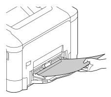
→ If a cap is in the long side of an envelope (western-style envelope #2, western-style envelope #6, or envelope DL), load the cap into the machine side.
